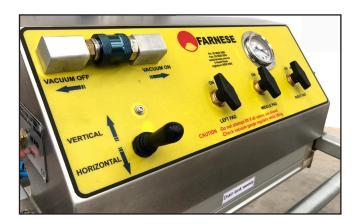
This essential piece of equipment is fitted with a pneumatic tilting piston which provides complete control of vertical and horizontal positions.
